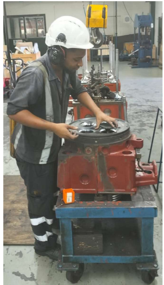
Performing engine overhaul
